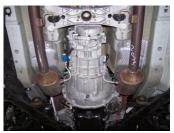
3. Now disconnect all 3 sensors on stock h-pipe with a 22mm wrench. Once you have done that, then unbolt the flanges at the stock manifolds and slide h-pipe out of rubber grommets. Save all stock hardware and clamps. You will re-use them later.
